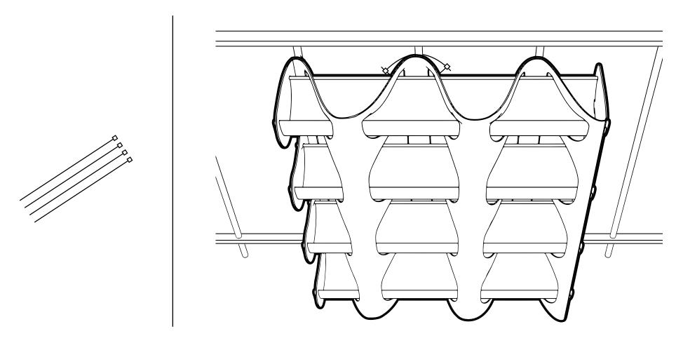
Attach the main frame to railings using the cable ties. Tip - if extra length is required, two cables can be joined together.
