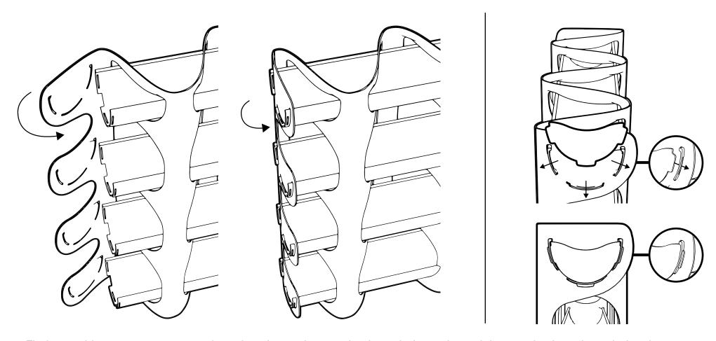
Find something or someone to push against. Insert the troughs through the end panel. Insert tab wings through the slots in the trough ends projecting through. Make sure each of the three wings on tabs are fully through. Repeat on other side.
