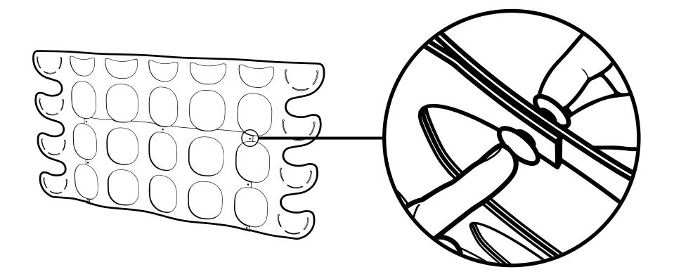
Locate all 7 rivets securing the smaller support panel to the main frame. Push rivets from both sides to snap them together to fix both components of main frame.
